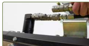
Hydraulisk snabbkoppling (standardutrustning)
