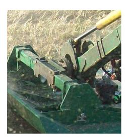
Before fitting the PTO for the first time it may be necessary to adjust the length. There should be maximum engagement of the sliding tubes without bottoming at the shortest operation position. To check, first connect the mower to the vehicle.
