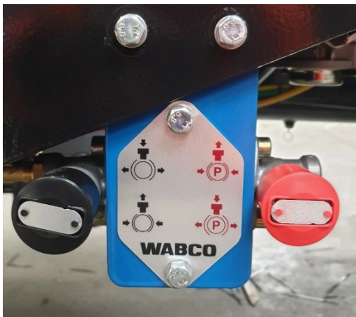
Diagram 4-3: Spring parking brakes control valve
